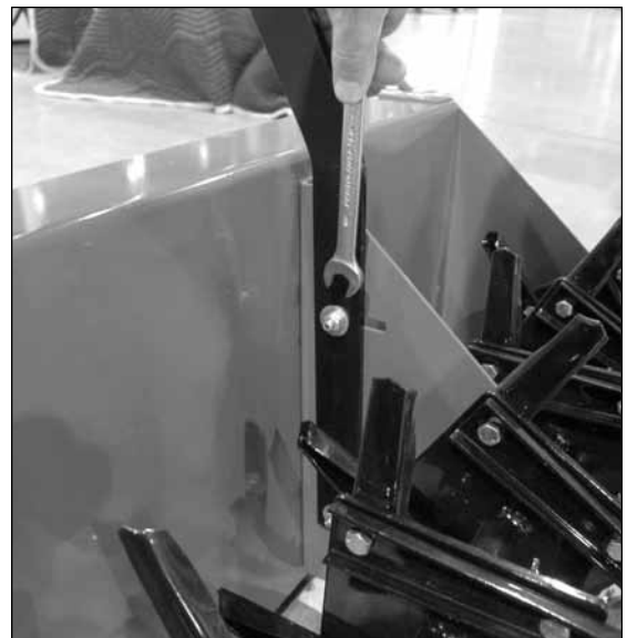
TONGUE BEING ASSEMBLED TO UNIT
