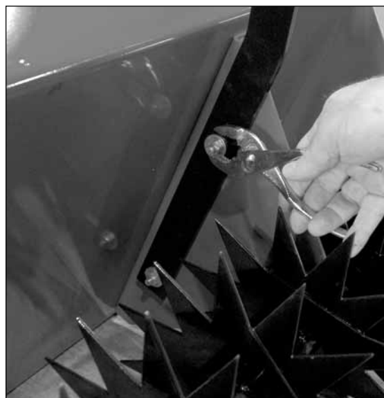
TONGUE BEING ASSEMBLED TO UNIT
