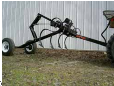
Properly installed S-Tines on the RMII
