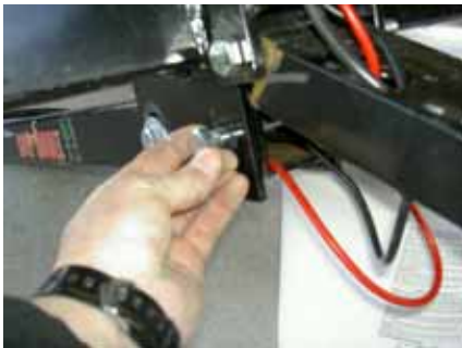
Bolt inserted in slotted tongue receiver
