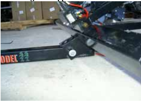
Bolt inserted in slotted tongue receiver
