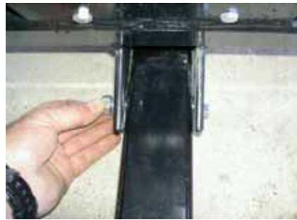
Nut being placed on bolt going through slotted tongue receiver
