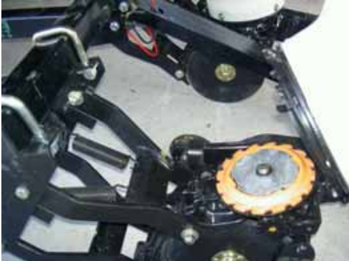
Pivot the seed hopper back to tighten down bolts
