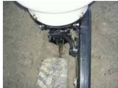
You should notice seed in the cut slot in the soil just before the packer wheel covers the seed.
