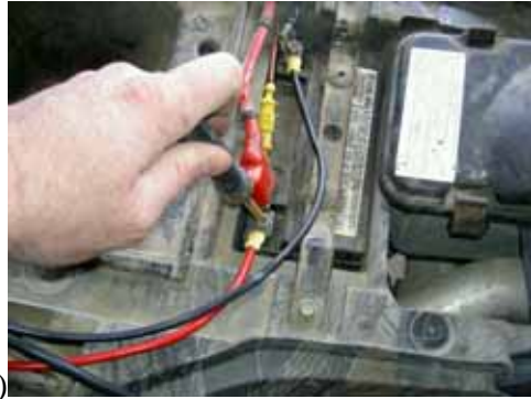
Secure electrical leads to your ATV battery
