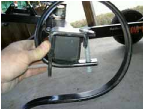
Slide the S-Tine bracket over the tool bar
