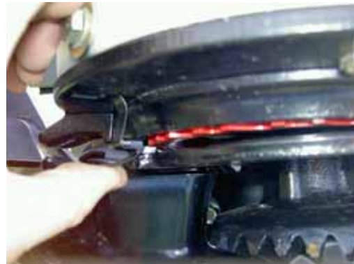
Lock the seed hopper down to the bottom of drive
