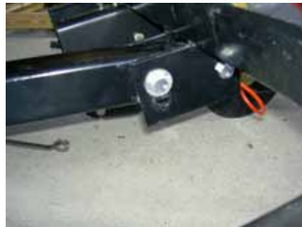
Nut being placed on bolt going through slotted tongue receiver
