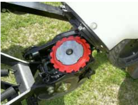
Seed plate in place on plate drive
