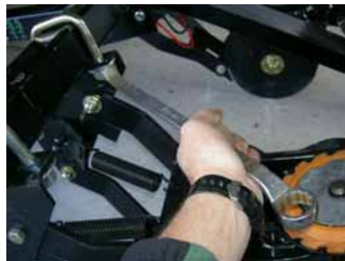
Tighten down bolts with a 15/16 wrench
