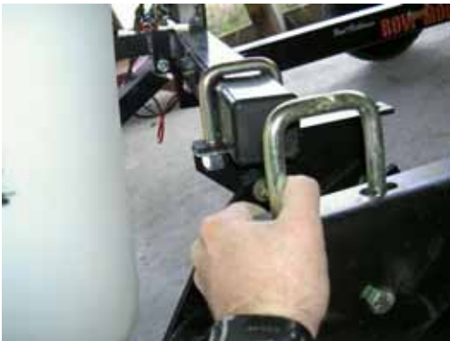
Slide the attached U-Bolts over the RM tool bar
