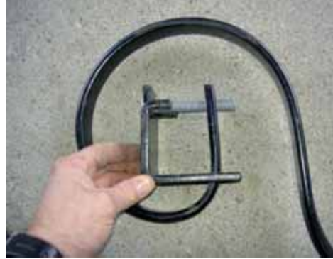
Place the bracket and bolt over the S-Tine
