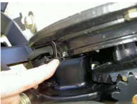
Completely locked over seed plate drive
