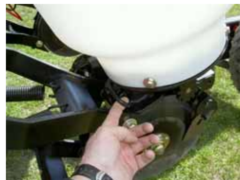
Lock the spring loaded pin to secure seed hopper
